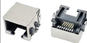
Side Entry Unshielded 8P 1X1 Port Sink-type Modular Jack, Stamp Pin, SMT Type w/o LED
