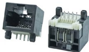
Side Entry Unshielded 8P Single Port Modular Jack, Round Pin, DIP Type
